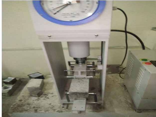
Figure - 9 flexural testing test set up
