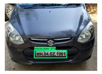
Similarly, the ROI of license plate is then extracted as an image as shown in the figure below. This extracted image is then passed for character recognition.
