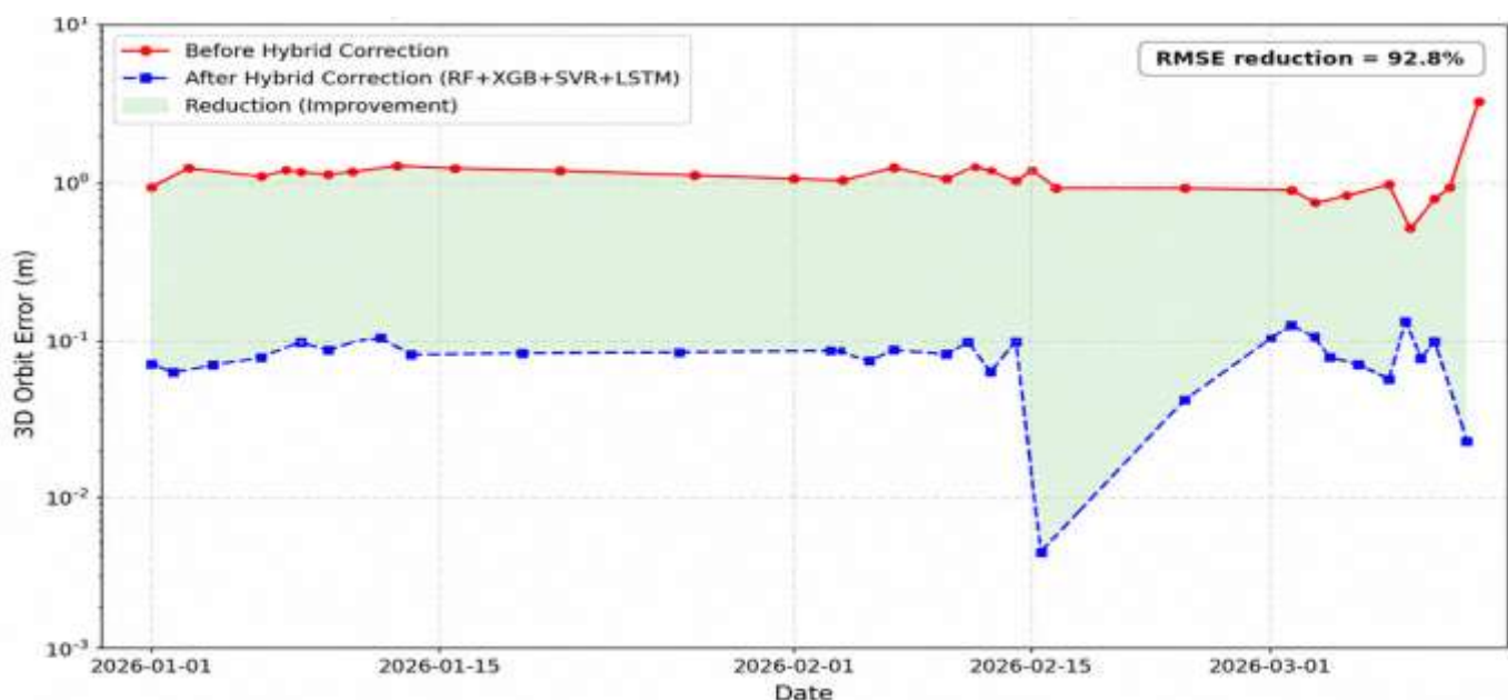
Figure 6. Temporal comparison of GEO 3D orbit error before and after staged hybrid correction, January to March 2026.
