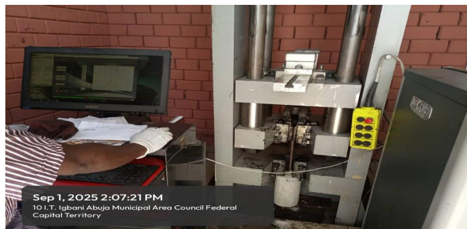
Figure 3. Post -installed Concrete Sample Fixed to Model and the applied load and corresponding displacement were continuously recorded by the UTM data-acquisition system
