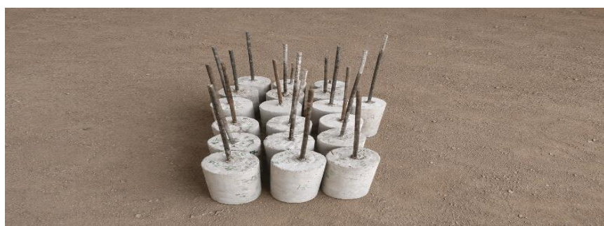
Figure 2. Bar Installed in Drilled Holes with Adhesive as Binding Agents
