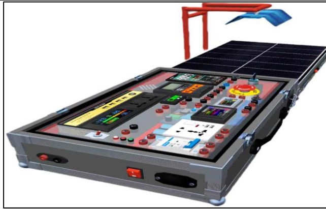
Fig. 7 Isometric View of the Photovoltaic System Trainer in Set-up Position
