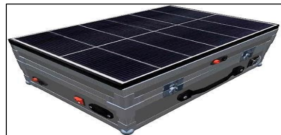
Fig. 6 Isometric View of the Photovoltaic System Trainer in Close Position
