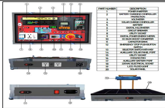
Fig. 2 Orthographic View with Major Parts of the Photovoltaic System Trainer
