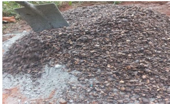
Figure 2: PKS concrete mix
