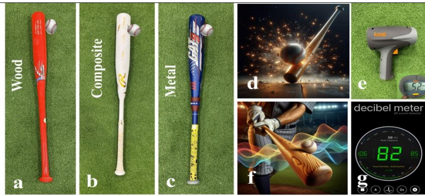
Figure 1. The bats used for experimental data collection; a) wood, b) composite, c) metal bats with their plausible interfaces with the baseball, d) Artificial intelligence (AI) generated drawing depicting the trampoline effect upon bat-ball collision, e) employed speed gun (insert shows measured speed), f) AI generated drawing demonstrating the acoustic effect using Copilot and g) screen shot of a decibel meter reading with iPhone Prox max 15.
