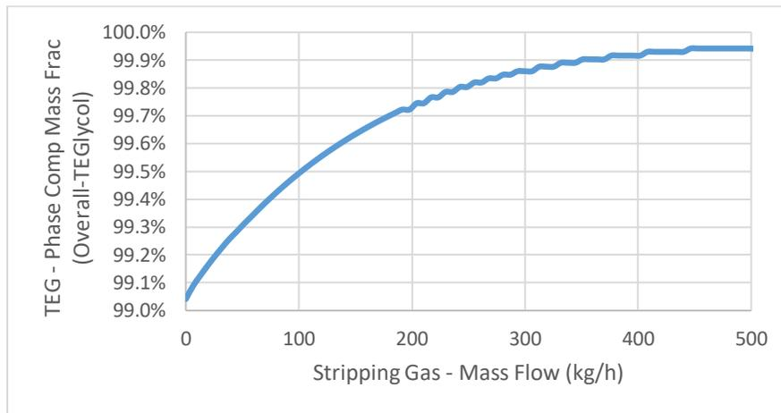
Figure 30: TEG purity vs. stripping gas mass flow
