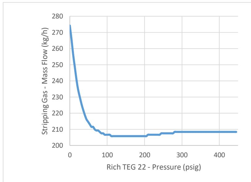
Figure 22: Stripping gas amount required for 99.75% purity of TEG vs. the flash tank operation pressure
