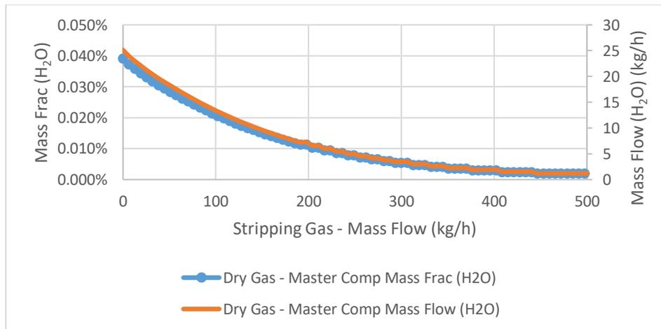
Figure 27: Dry Gas water content vs. stripping gas mass flow
