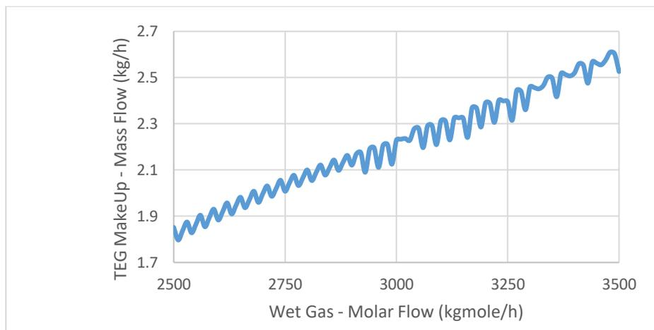
Figure 13: TEG loss vs Wet Gas flowrate
