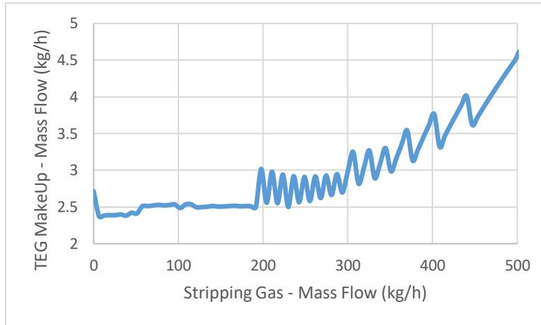
Figure 29: TEG loss vs. stripping gas mass flow
