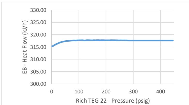
Figure 20: TEG boiler duty vs. the flash tank operation pressure
