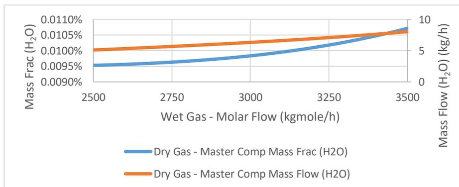
Figure 11: Dry gas water content vs. wet gas flow rate
