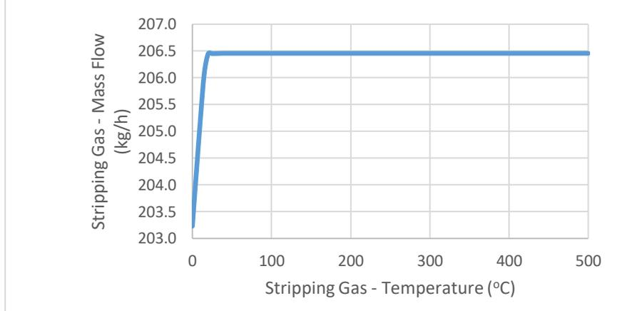
Figure 26: Stripping gas amount required for 99.75% purity of TEG vs. stripping gas temperature
