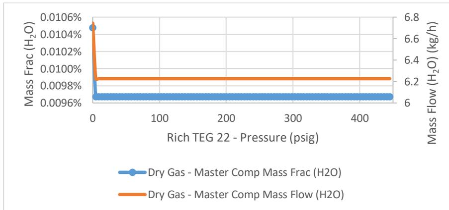
Figure 19: Dry gas water content vs. the flash tank operation pressure
