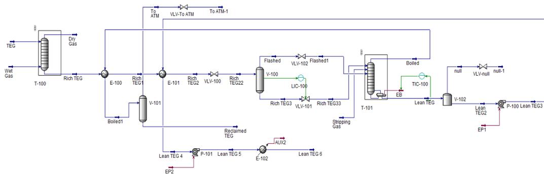
Figure 2: Dynamic simulation of dehydration unit
