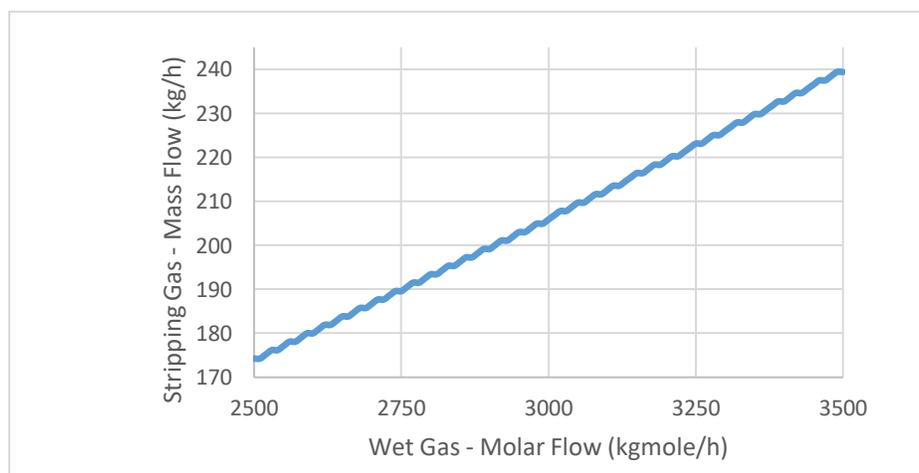
Figure 14: Stripping gas amount required for 99.75% purity of TEG vs. wet gas flow rate
