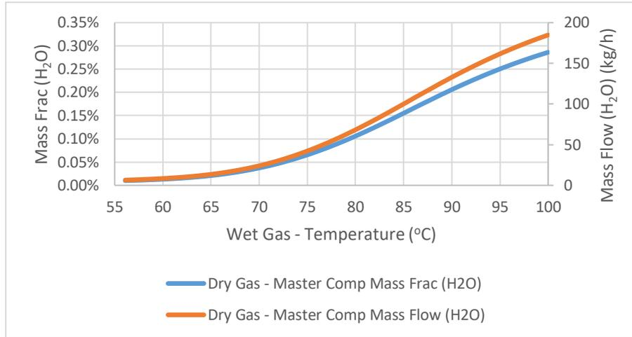
Figure 15: Dry gas water content vs. wet gas feed temperature
