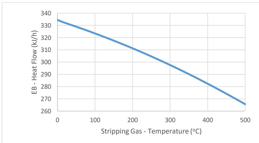
Figure 24: TEG boiler duty vs. the stripping gas temperature
