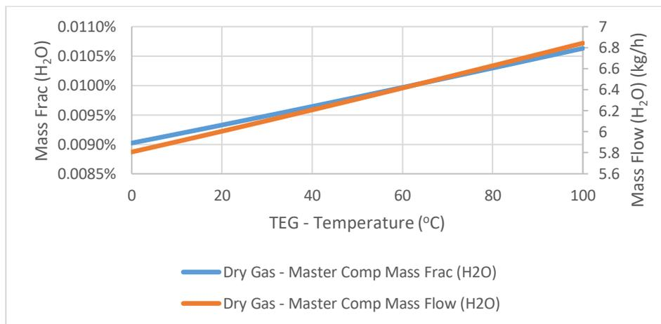
Figure 7: Dry gas water content vs. TEG feed temperature
