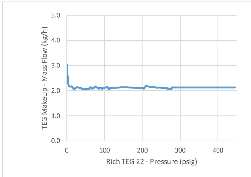
Figure 21: TEG loss vs the flash tank operation pressure
