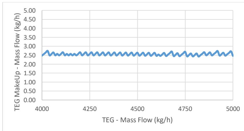
Figure 5: TEG loss vs. TEG circulation rate
