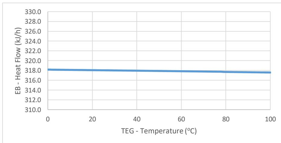
Figure 8: TEG boiler duty vs. TEG feed temperature
