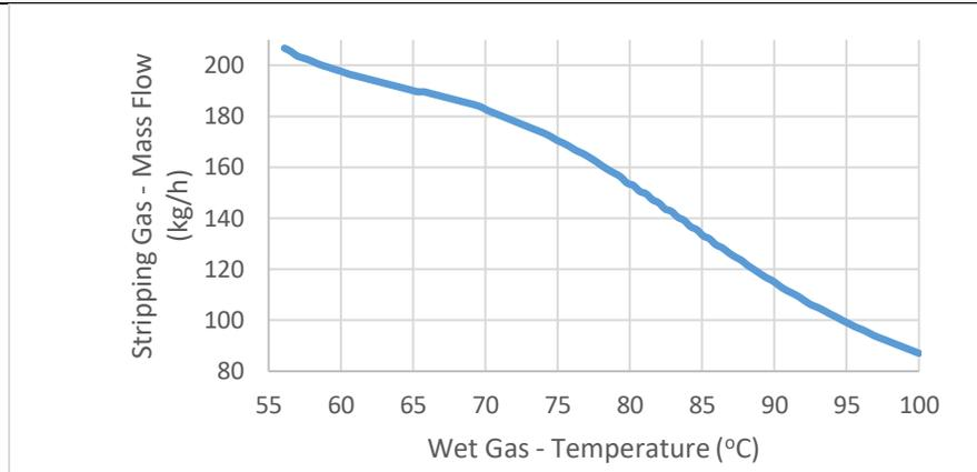
Figure 18: Stripping gas amount required for 99.75% purity of TEG vs. wet gas feed temperature
