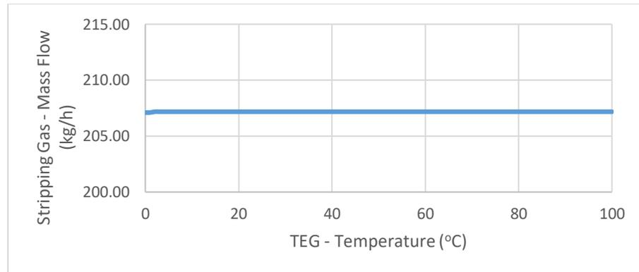
Figure 10: Stripping gas amount required for 99.75% purity of TEG vs. TEG feed temperature
