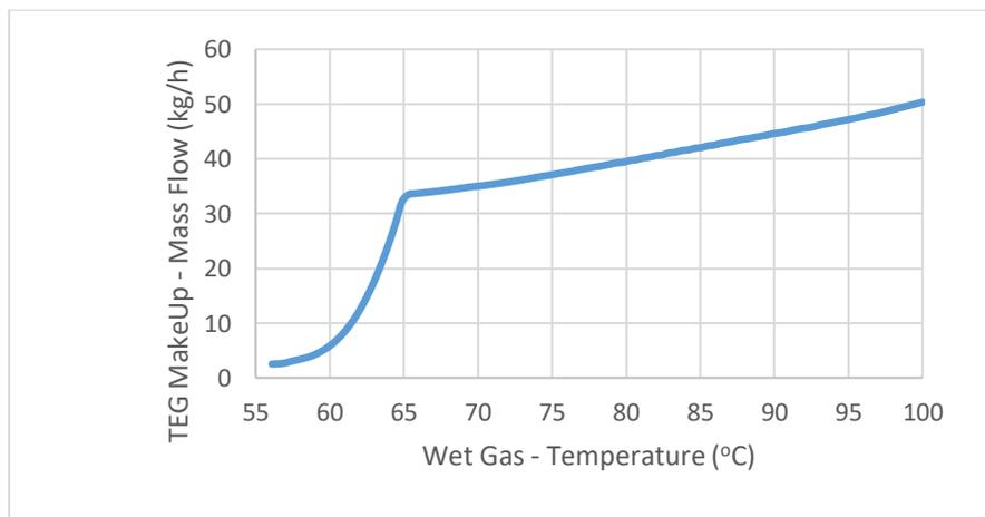
Figure 17: TEG loss vs. wet gas feed temperature
