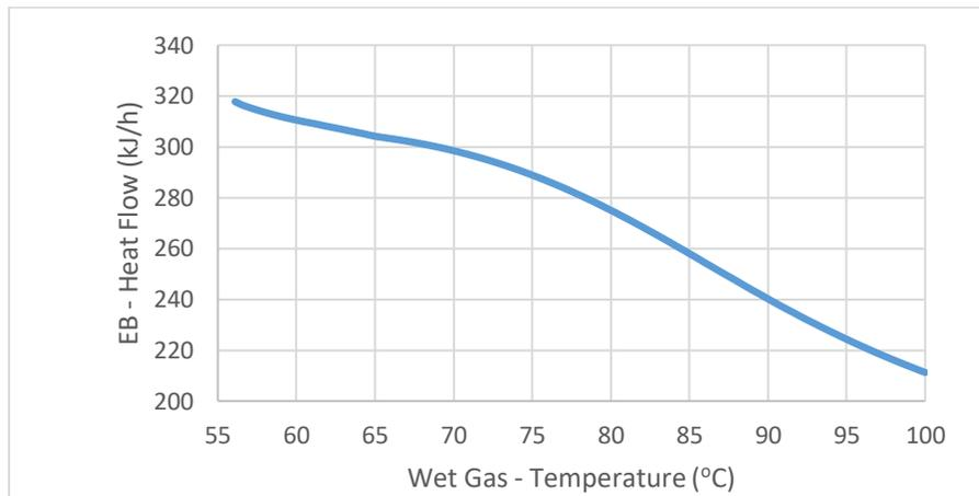
Figure 16: TEG boiler duty vs. wet gas feed temperature
