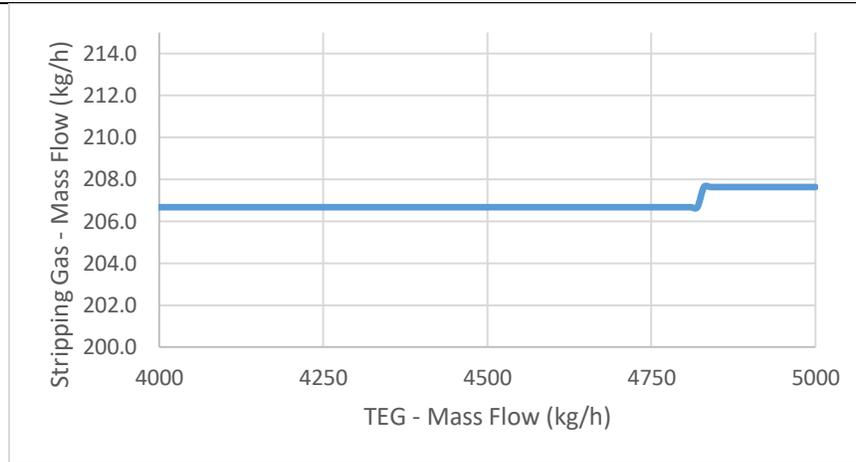
Figure 6: Stripping gas amount required for 99.75% purity of TEG vs. TEG circulation rate
