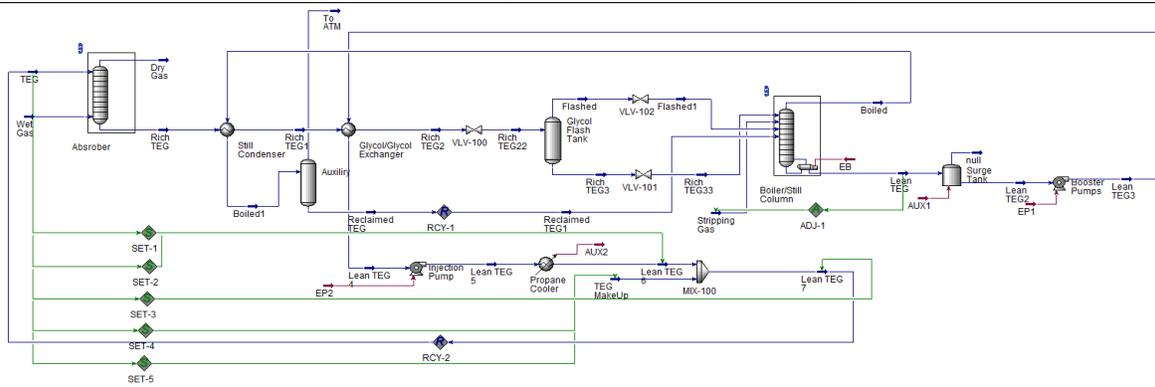
Figure 1: Steady State simulation of dehydration unit
