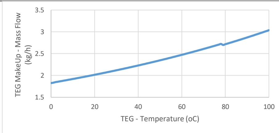
Figure 9: TEG loss vs. TEG feed temperature
