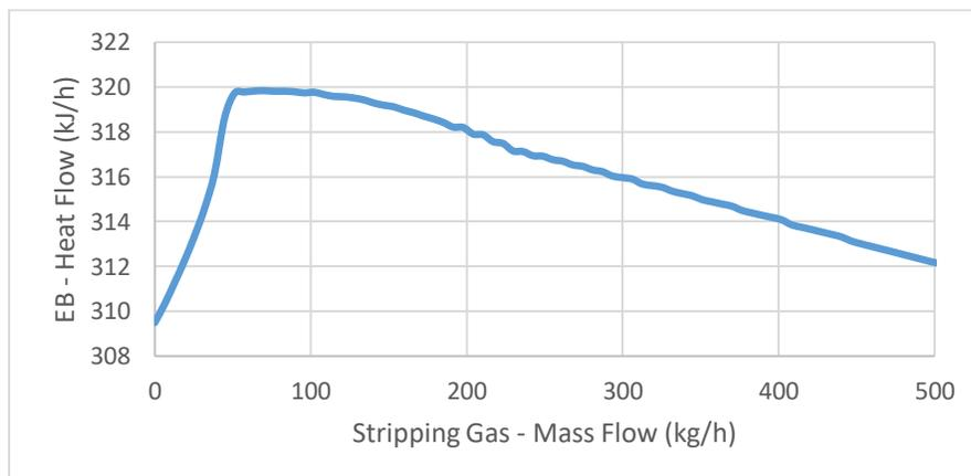
Figure 28: TEG boiler duty vs the stripping gas mass flow
