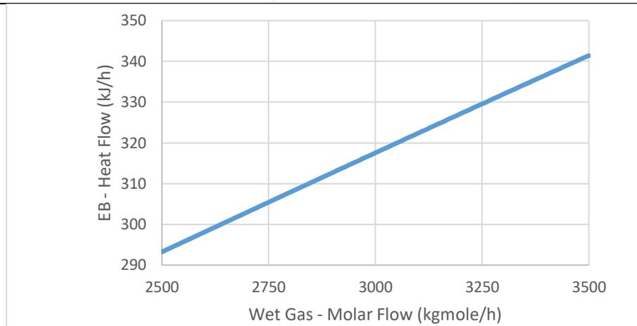
Figure 12: TEG boiler duty vs. wet gas flow rate
