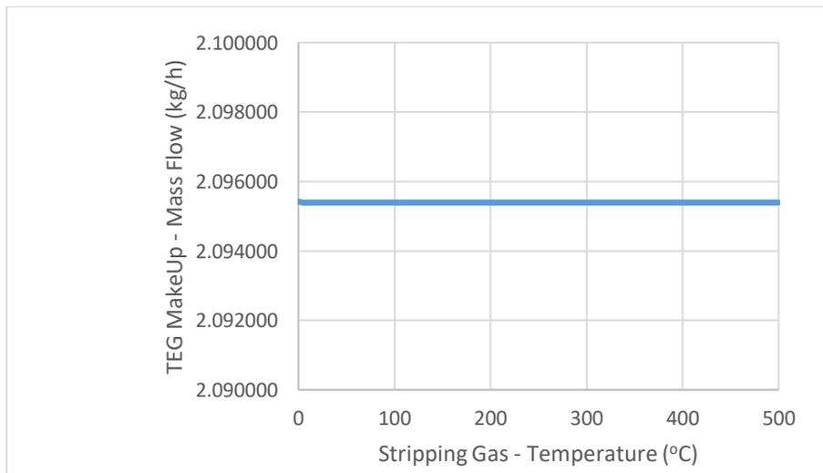
Figure 25: TEG loss vs stripping gas temperature
