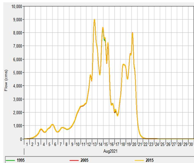
Figure 12: Hydrograph for HRS Catchment Outlet
