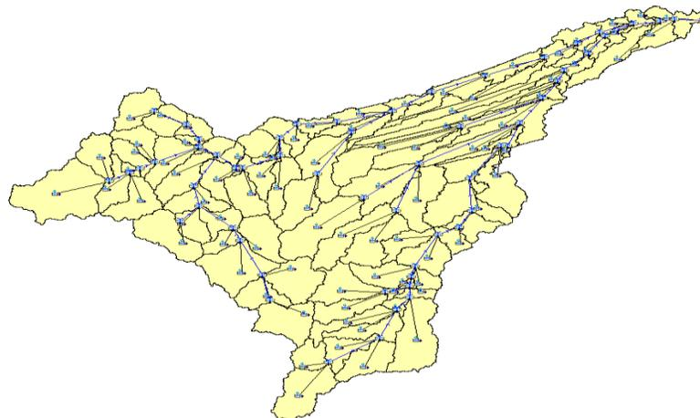
Fig. 13: Hydrologic modeling of the HRS using HEC-HMS
