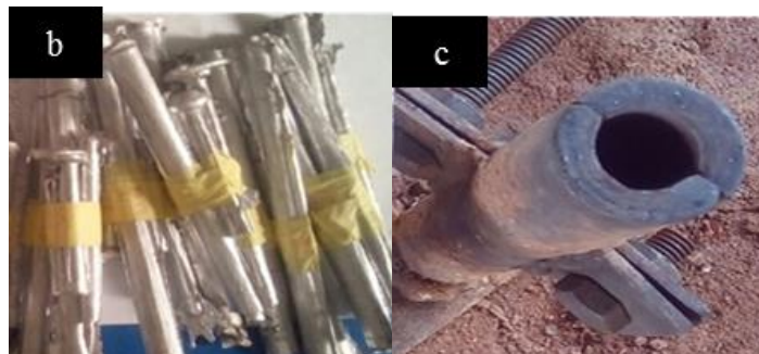
Fig. 1. (b) As-cast AA6063/GNSA composites, (c) Fabricated permanent mould
